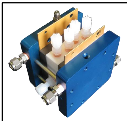
BT-112 – Shown with SAI Test Fixture
